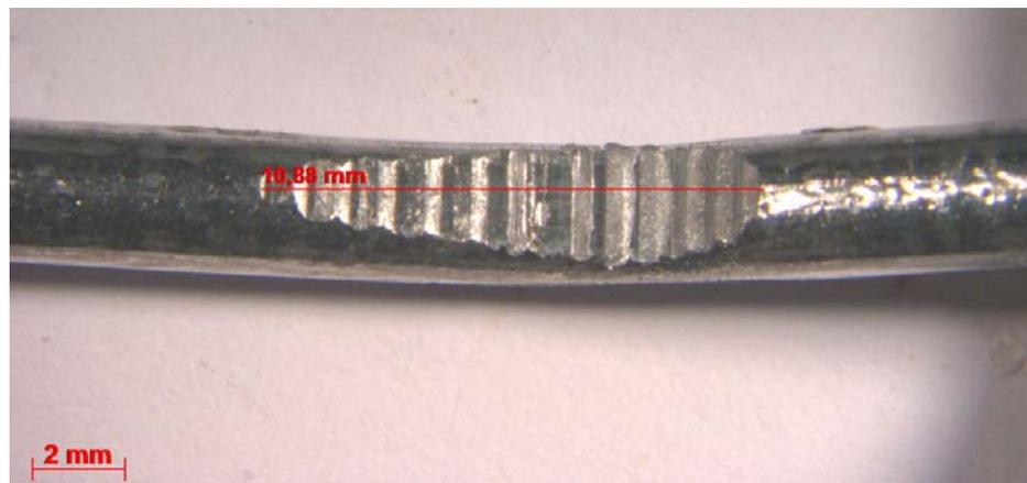
Photo 6: Deformation of crop wire Crapal 3.15 mm in the clamping mechanism of Gripple GP90, after performing a static load test.
