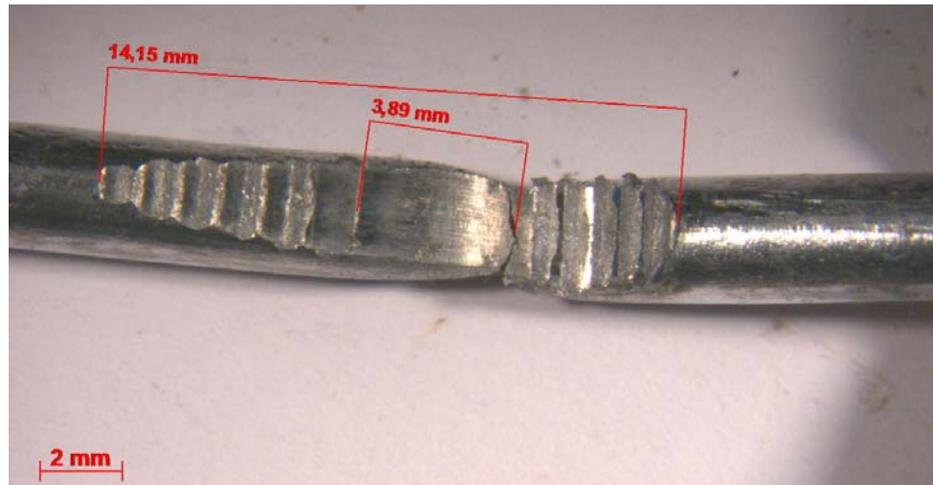
Photo 5: Deformation of crop wire Crapal 3.15 mm in the connection with Gripple GP90, after breakage of the wire.
