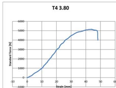
Figure 1: chart of a static load test on the connection between Gripple GP90 and crop wire galvanized 3.80 mm.
