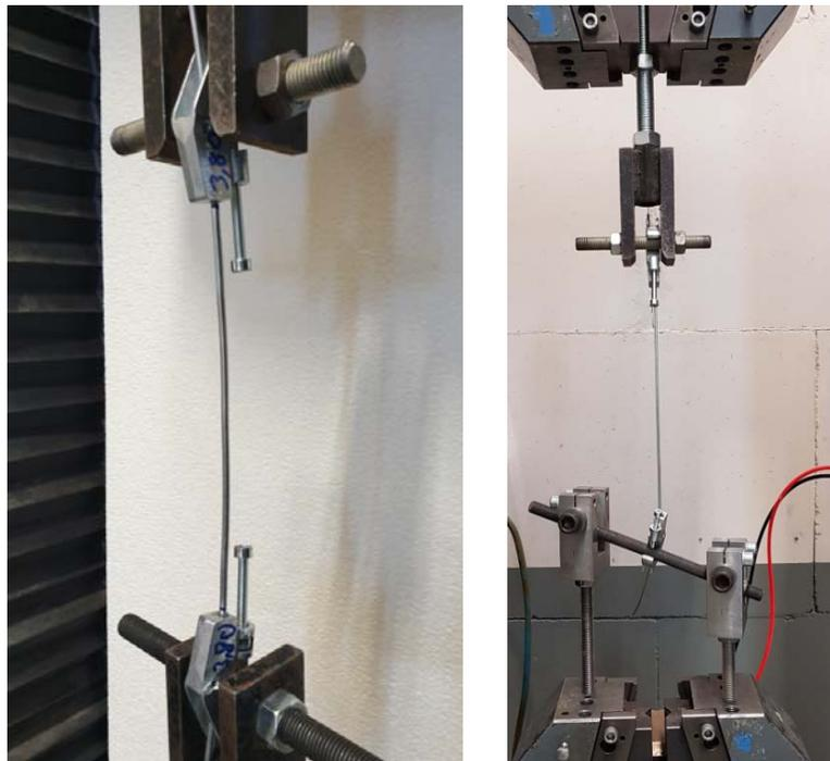
Photo 2 and 3: Crop wire connection with Gripple GP90 in the test setup for static load testing. On the left the right angled connection of the crop wire, on the right the connection of the crop wire at an angle of 20 degrees.
