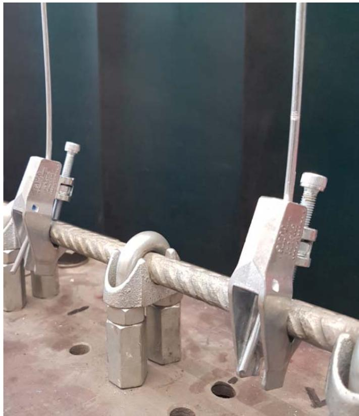
Photo 1: connection of crop wires to steel rod 14 mm with Gripple 90GP in the test setup.
