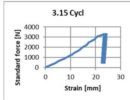
Figure 2: chart of a test with alternating load on the connection between Gripple GP90 and crop wire Crapal 3.15 mm.
