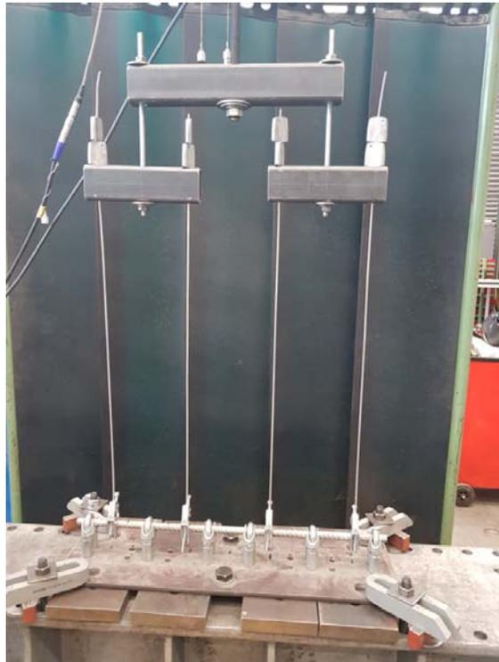
Photo 4: Crop wire connection with Gripple GP90 in the test setup for testing the resistance to alternating load.
